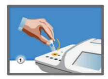
The system is designed to be used by anyone, without the support of skilled staff. The analysis methods are easier than the traditional ones and can be performed in few steps: 1 Adding the sample volume to the pre-vialed reagent. 2 Following the displayed instructions and if there is ever a doubt, the **HELP function** will lead you through the process. 3 Results are automatically calculated, displayed and printed.
