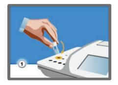
Each test is performed dispensing in the cuvette containing the buffer a determined amount of the sample. Thanks to the reagents created on purpose, it is generated a colorimetric reaction. The result of the test is printed immediately after the elaboration of the photometric reading, in its unit of measure.
