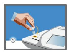
Each test is performed dispensing in the cuvette containing the buffer a determined amount of the sample. Thanks to the reagents created on purpose, it is generated a colorimetric reaction. The result of the test is printed immediately after the elaboration of the photometric reading, in its unit of measure.
